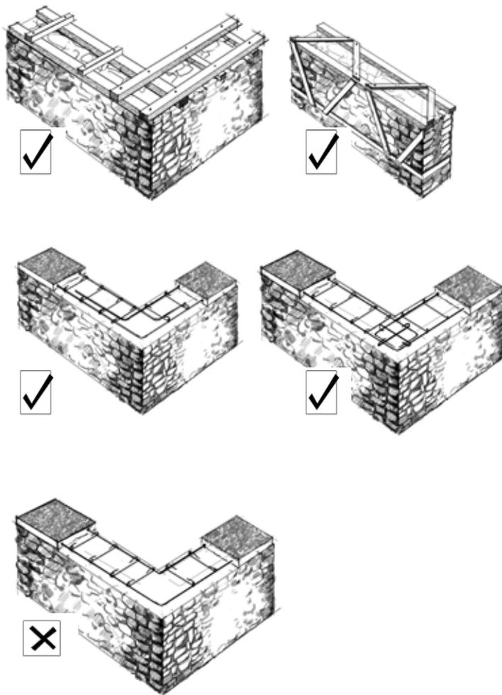
Figure 3.14 Recommended detailing of timber and RC bands (adapted from: T. Schacher and C.V.R. Murty)
