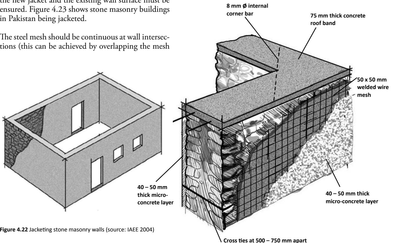
Figure 4.22 Jacketing stone masonry walls (source: IAEE 2004)
