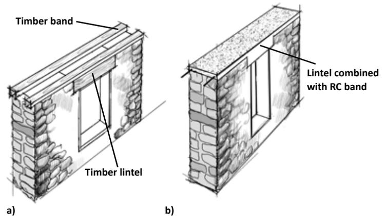
Figure 3.13 Combining floor/roof and lintel band: a) timber band, and b) RC band
