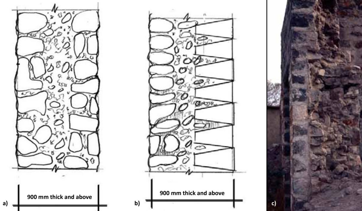
**Figure 1.28** Stone masonry walls in Maharashtra, India: a) an uncoursed random rubble stone masonry wall (source: CBRI 1994); b) a semi-dressed stone wall with an exterior wythe built using wedge-shaped dressed stone (Source: CBRI, 1994), and c) an example of a semi-dressed stone wall (photo: S. Brzev)
