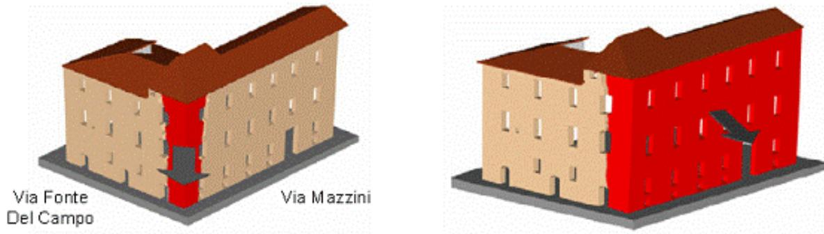
**Figure 2.26** Rendered images of a building damaged in the 2002 Molise (Italy) earthquake: a) the stone masonry construction is damaged at the corner resulting in a loss of gravity support; b) a façade falls away from the floor and roof diaphragms (source: Maffei et al. 2006)
