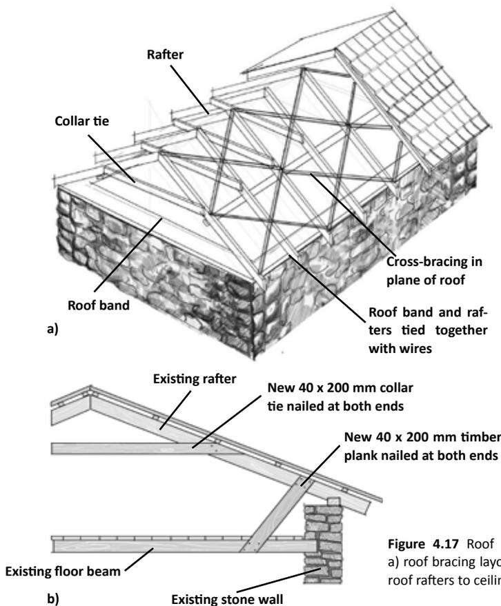
Figure 4.17 Roof bracing details: a) roof bracing layout, and b) tying roof rafters to ceiling joists
