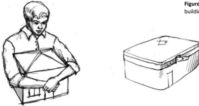
Figure 3.7 A seismic band acts like a belt (adapted from: GOM 1994)
