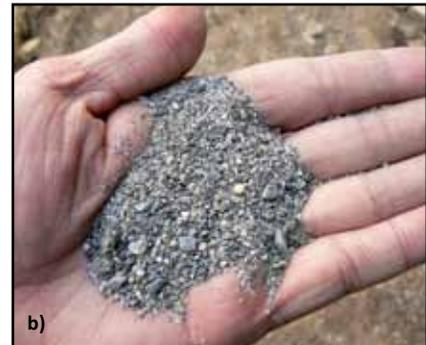
Different types of sand and their uses are illustrated in Figure 3.42. If the sand is too coarse, small pebbles must be sieved out. These pebbles could be added to aggregate for concrete construction. Sand from the sea or ocean should not be used due to the presence of salt (chlorides), which causes corrosion of steel reinforcement.
